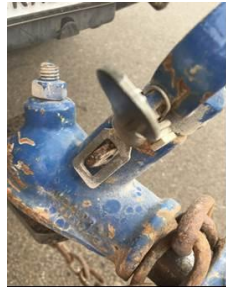
Pins and chains secured
